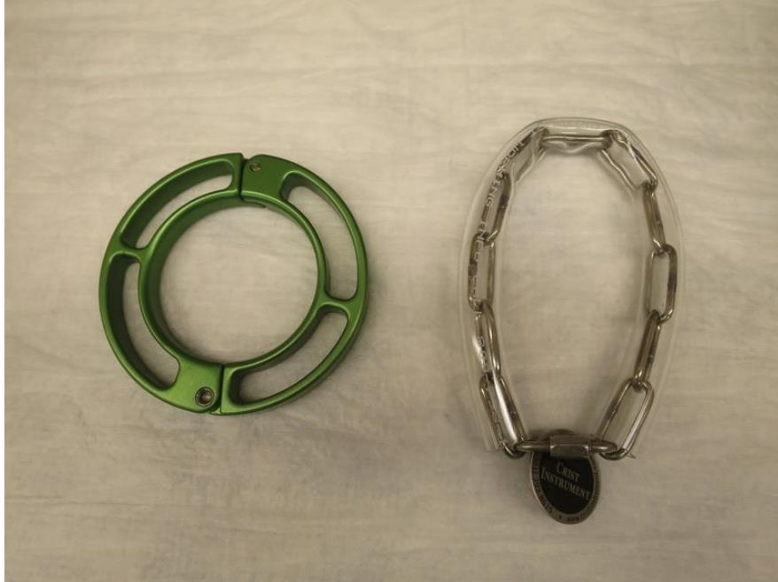
Figure 3. Primate collars. Left: rigid aluminum collar. Right: chain-link collar encased by flexible PVC.
