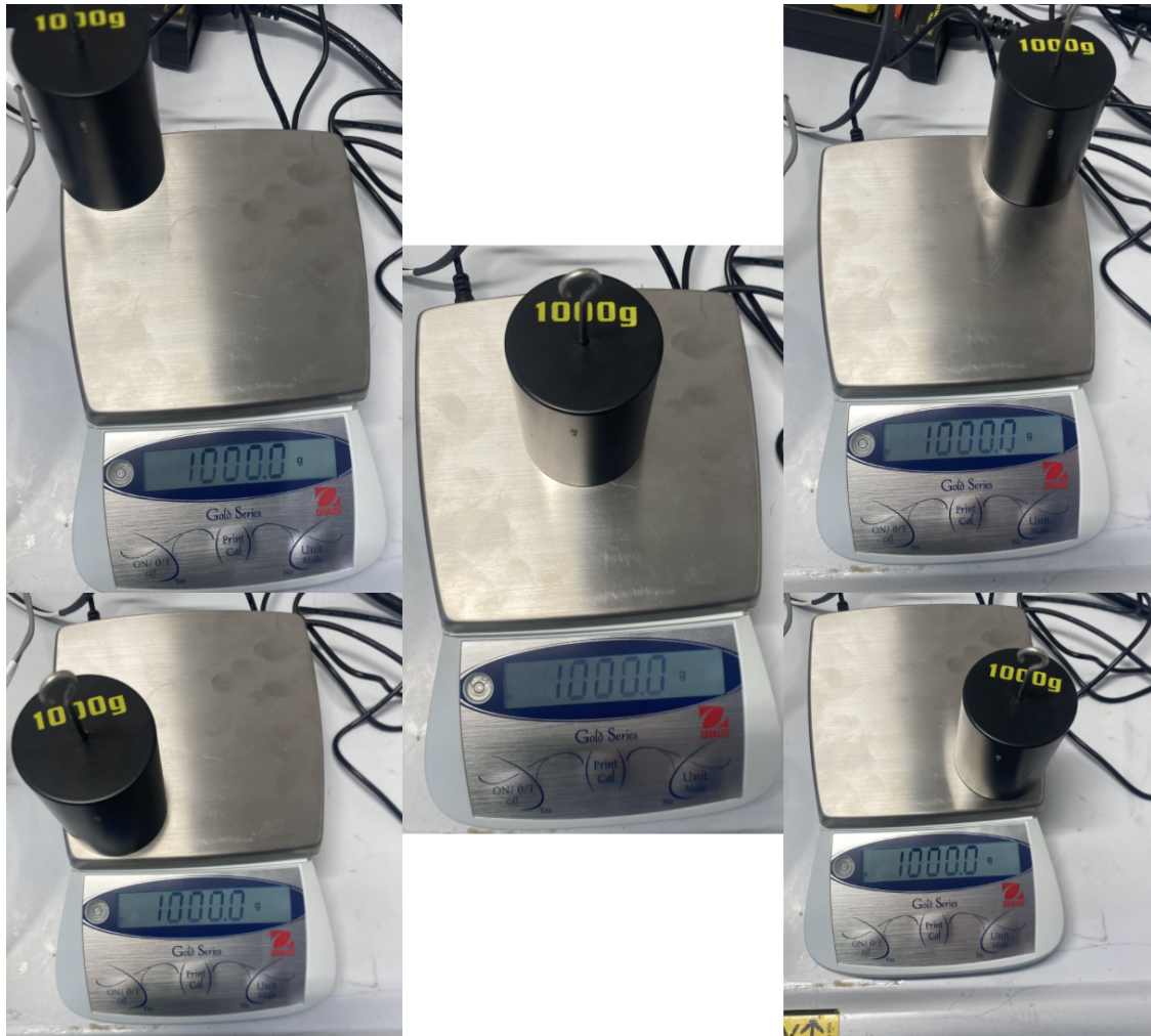
Figure 7.1: Five loading cases on the OHAUS TAJ 4001 scale showing it accurately reads mass everywhere on the loading plate.
