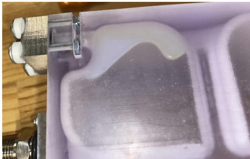
Figure 6.18: Hot glue in storage tank
