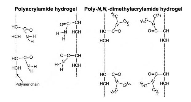
Polymer Structure and Water Absorption Mechanism\_Hydrogel
