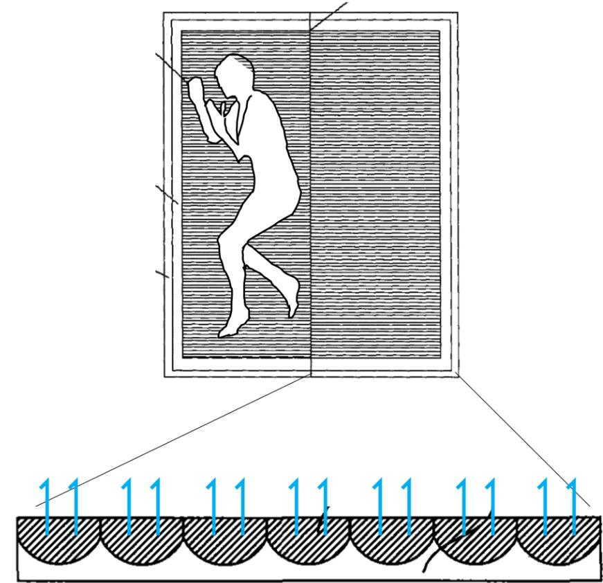
Without human body atop: Liquid within bamboo evaporates and cools down the sheet
