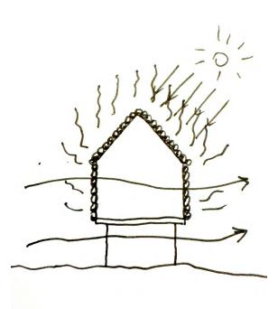
Diurnal Water Cycle for Passive Cooling
