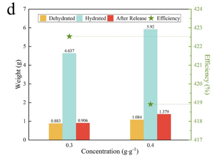
“In addition, LCP hydrogels can absorb 1.93g/g water overnight (13h) at RH 90% and easily release up to 99.38% of the absorbed water via the photothermal effect under 500W/m<sup>2</sup> light. It is estimated that the daily water yield can reach up to approximately 2.56kg/kg\*day with three cycles.”
