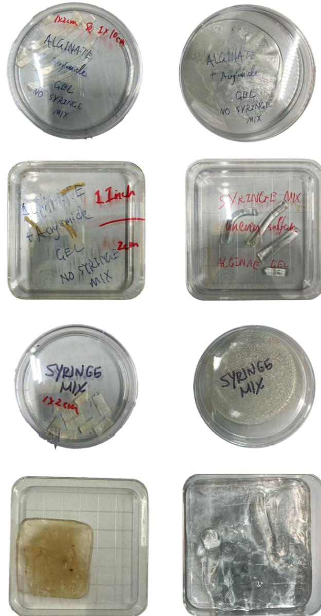
Acrylamide-Alginate DN Gel samples of different scale and shape
