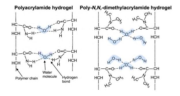
Polymer Structure and Water Absorption Mechanism\_Hydrogel
