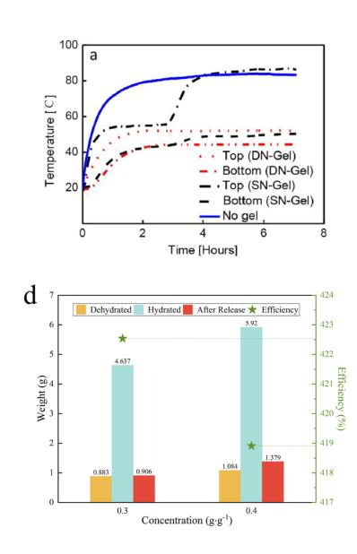
"In addition, LCP hydrogels can absorb1.93g/g water overnight (13h) at RH 90% and easily release up to 99.38% of the absorbed water via the photothermal effect under 500W/m2 light. It is estimated that the daily water yield can reach up to approximately 2.56kg/kg\*day with three cycles."
