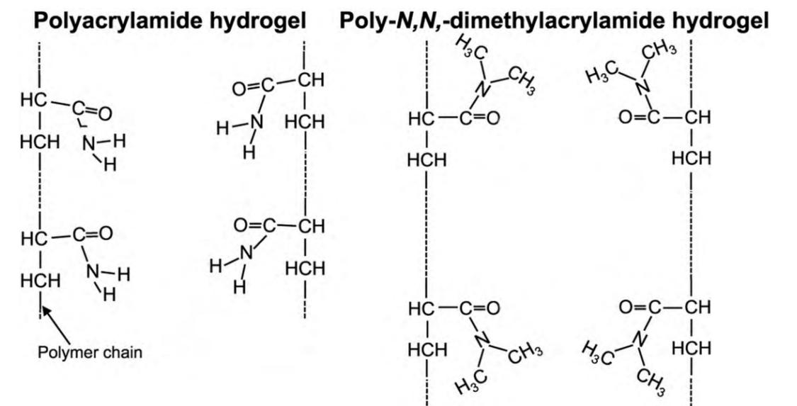
Polymer Structure and Water Absorption Mechanism\_Hydrogel
