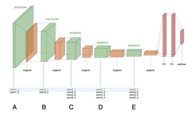
Figure 1. VGG 19 Convolutional Neural Network.
