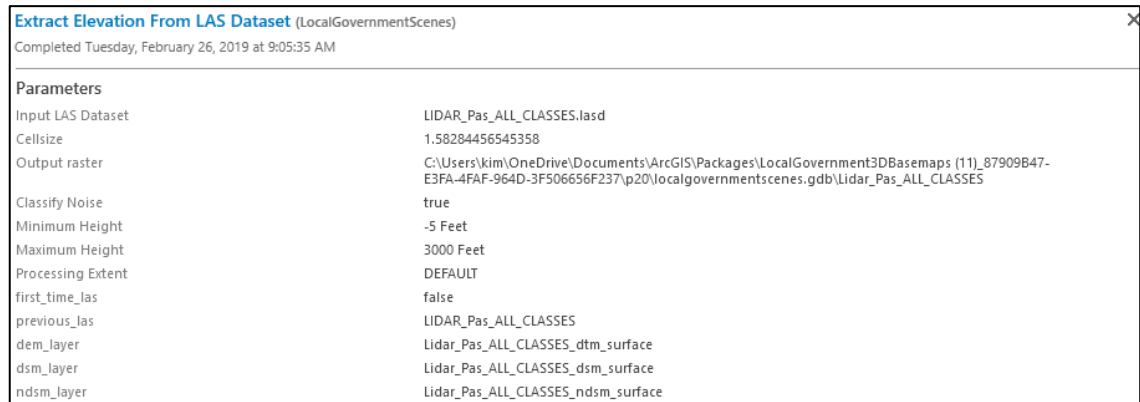
Figure 63. Parameters used to extract elevation from LAS Dataset.
