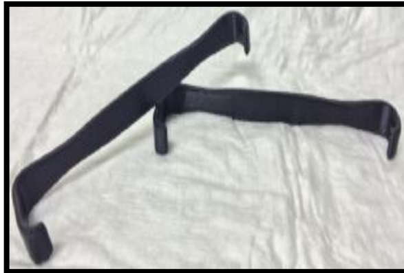
Figure 34. 3D-printed polylactic acid Army-Navy surgical retractor (Rankin et al., 2014)
