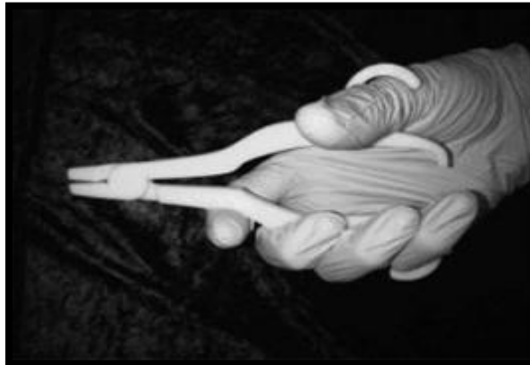
Figure 35. 3D-printed acrylonitrile butadiene styrene needle driver (Kondor et al., 2013)
