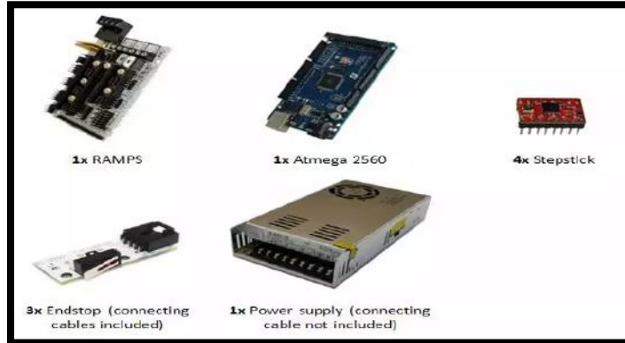
Figure 18. The essential electronic components for the RepRap device (RepRap Bill of Materials)
