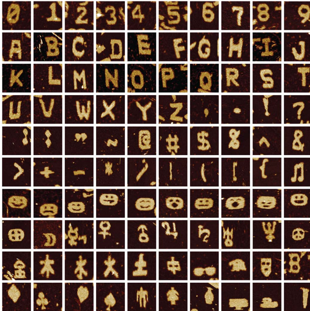
Figure 2.4 Complex shapes designed using a “molecular canvas.” AFM images of 100 distinct shapes, including 26 capital letters for the full English alphabet, 10 Arabic numerals, 23 punctuation marks and other standard keyboard symbols, 10 emoticons, 9 astrological symbols, 6 Chinese characters, and various miscellaneous symbols. Image size, 150 nm × 150 nm.
