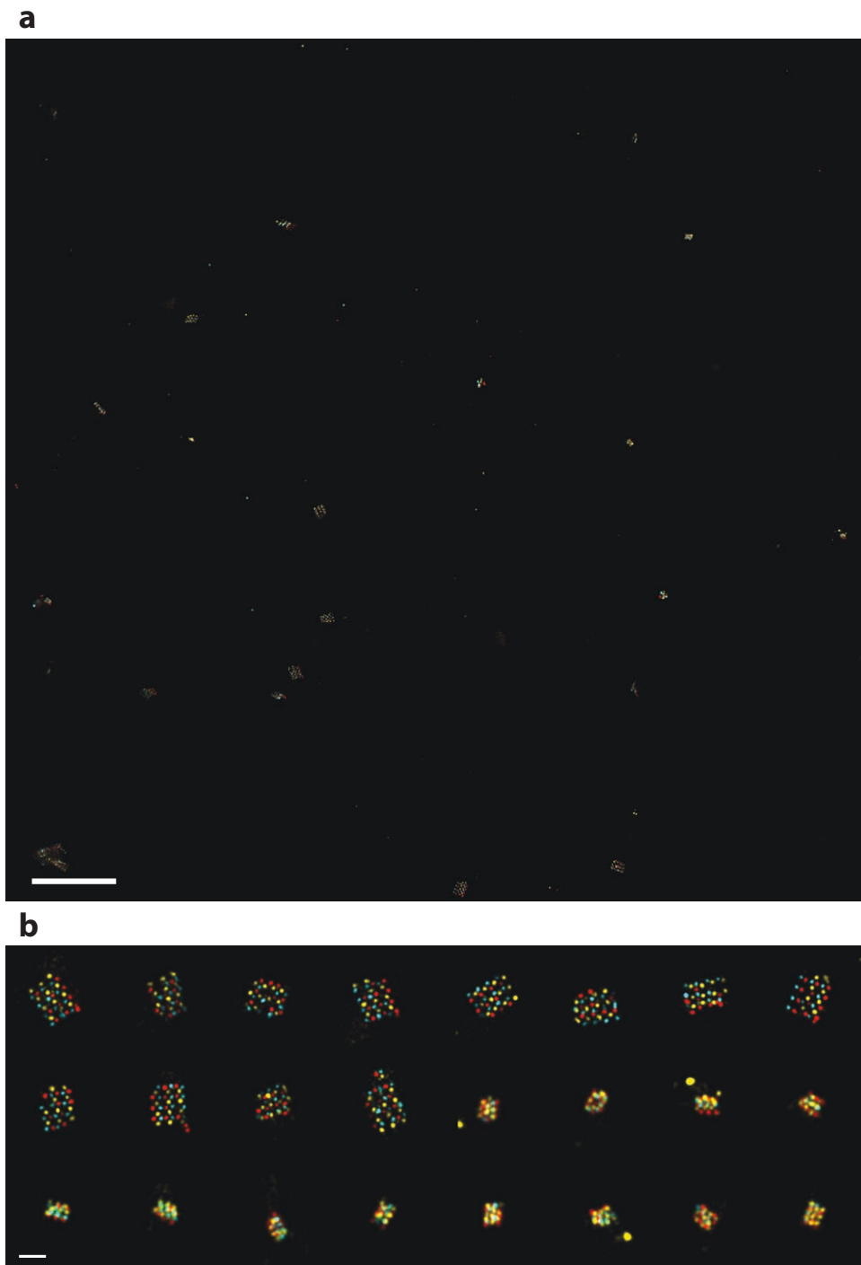
Figure S24. DMI super-resolution image of the three-colour drift and alignment marker (a) Overlaid three-colour large field of view image. (b) Examples of cropped single-molecule three-colour drift and alignment markers, and 5 nm grid samples of two kinds. DNA-PAINT movie was collected with \sim 1.0 \text{ kW/cm}^2 laser intensity, 2-3 nM imager strand, and 20,000 frames at 400 ms per frame for each colour channel. Scale bars (a) 500 nm, (b) 50 nm. See high resolution version of Supplementary Figure S24 as a separate supplementary image file.
