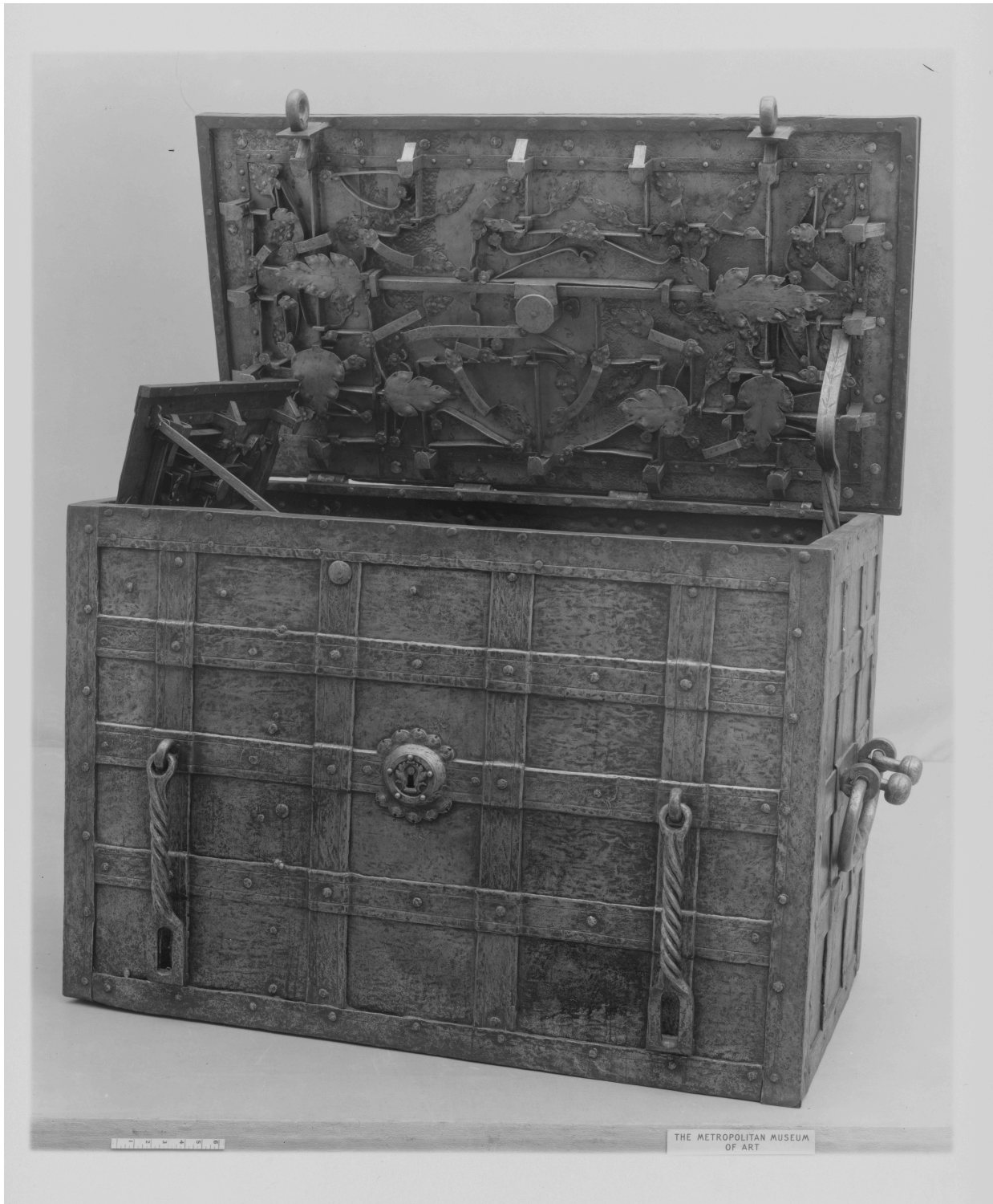
Figure 4.3: Steel strongbox, Nuremberg, (late 16th or early 17th century). Its elaborate locking mechanism consists of nine bolts and various leaf-shaped shields. Metropolitan Museum of Art. Accession number 90.13.1.
