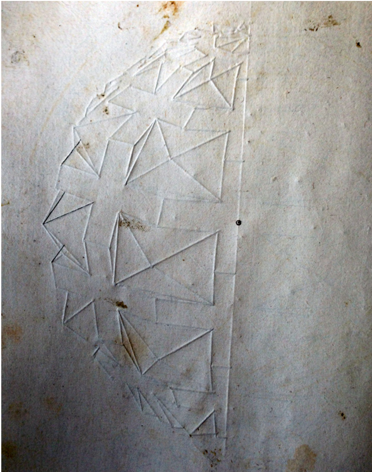
Figure 5.19: Verso side of a construction drawing for a geometrical model from Lorentz Stoer's Optica . Only half of the spherical form has been scored, due to its symmetry. Universitätsbibliothek Erlangen.
