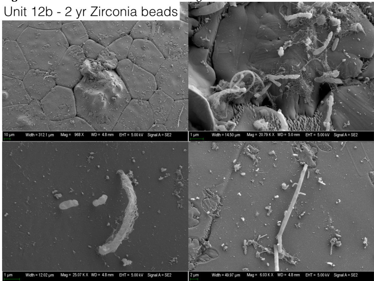
Figure D5. Zirconia bead surfaces showing microbial attachment.
