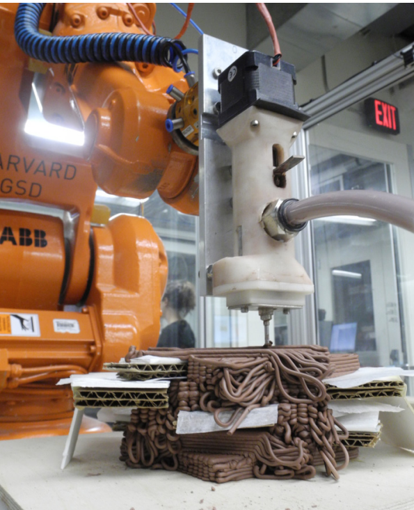
Fig 90. Accumulation of patterns with a clay extruder (here attached to a robot arm) creating Streamline objects. Photos by Kevin Hinz.
