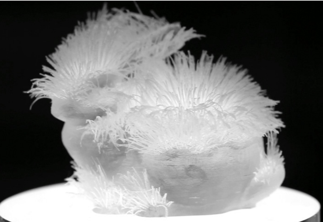
Fig 13. Cillia is a project of the MIT Media Lab group Tangible Media and allows “to 3D print hair-like structure on both flat and curved surfaces”. Description and photo by authors. http://tangible.media.mit.edu/project/cillia/
