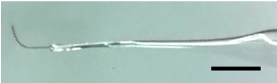
Figure 3. Wire tool used for removing embryos from the brood pouch. The tool shown here was made by inserting a tungsten wire into the narrow end of a Pasteur pipette and gently melting the glass to seal the wire in place, then using forceps to introduce a gentle curve into the wire. Other tools appropriate for removing embryos from the brood pouch include blunted forceps or a glass capillary with a sealed and smoothed end. Scale bar = 1 cm.
