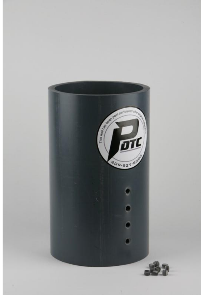
Figure 10. Example of 8 inch casing after perforation with 3/8 inch apertures (Stamoulis, 2011).
