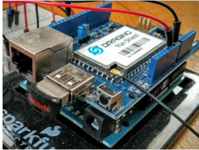
Figure 8 - Arduino Leonardo with YUN shield and USB drive installed
