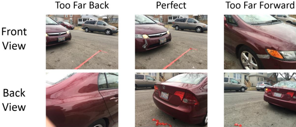
Figure 9. Single Meter Architecture Robustness. By having two cameras per meter, each facing in the opposite direction, the single meter architecture ensures that even when the vehicle is not positioned optimally, at least one meter will be able to capture and image of the vehicle license plate.
