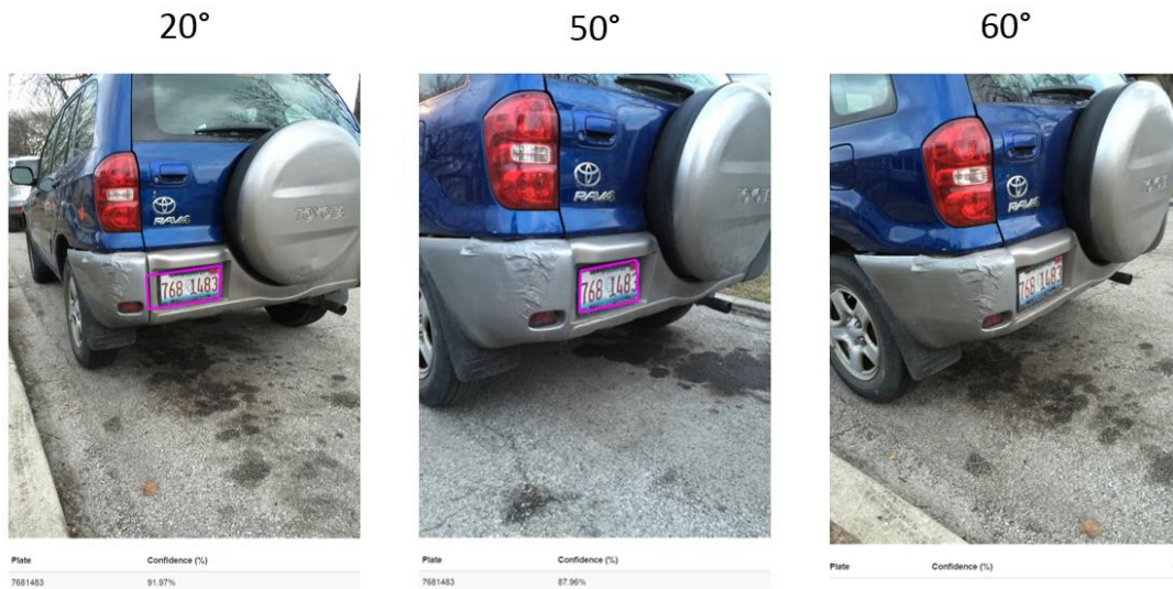
Figure 21. OpenALPR Evaluation. On average, the algorithm can tolerate up to 55° of perspective skew between the surface of the license plate and the camera.
