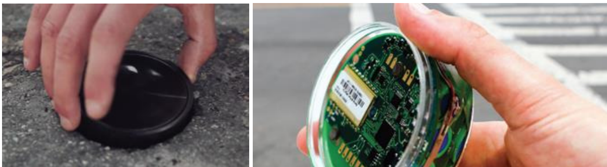
Figure 4. IPS Group Vehicle Detection Technology consisting of a sensor and transmitter that communicates with the corresponding single-space parking meter. The sensor requires a small hole in the ground of the parking space [4].
