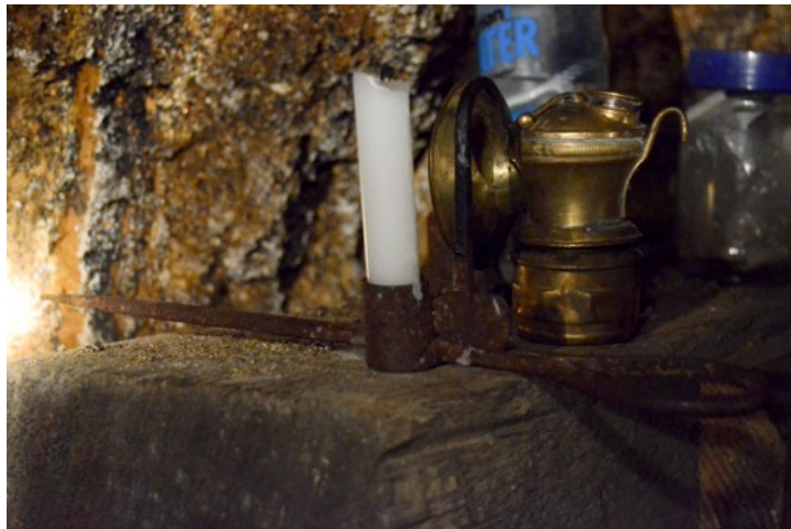
Figure 6.3. Miner's candlestick and candle, seen here next to a carbide head lamp, which replaced candles in the Butte Mines after 1912. (Photo taken by author at the World Museum of Mining, Butte, MT, May 18, 2012.)
